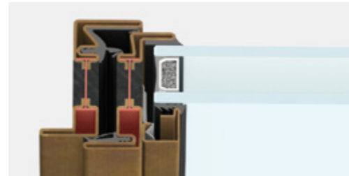
lateral section | frame section 47 mm
