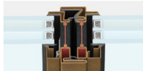
central section | frame section 62 mm
