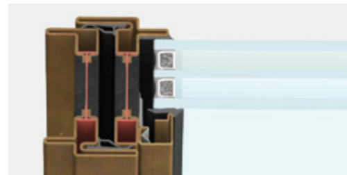
lateral section | frame section 47 mm
