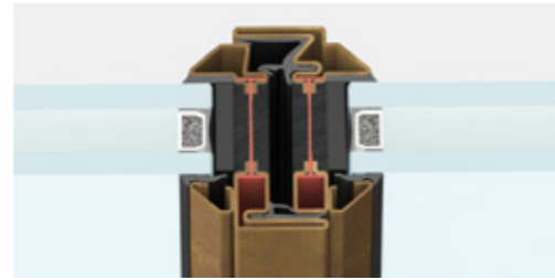
central section | frame section 62 mm
