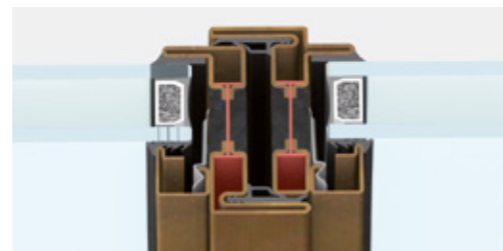
central section | frame section 62 mm
