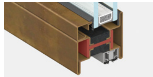
bottom rail | frame section 54 mm
