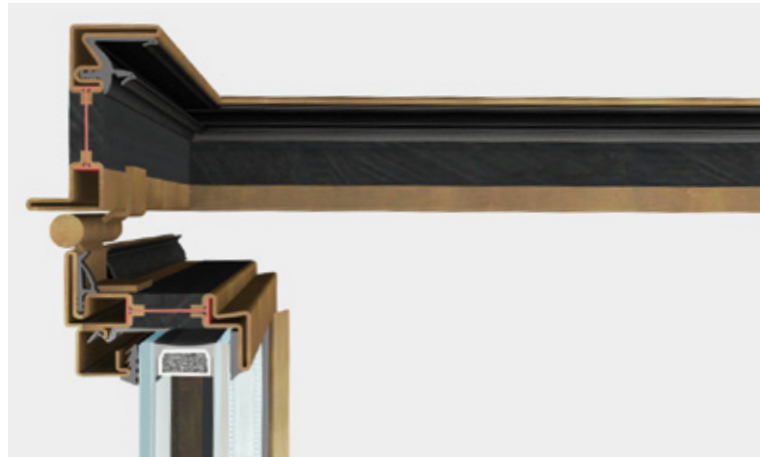
lower section | frame section 47 mm
