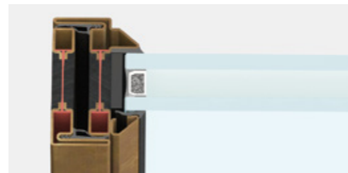
lateral section | frame section 47 mm
