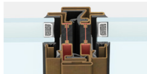
central section | frame section 62 mm
