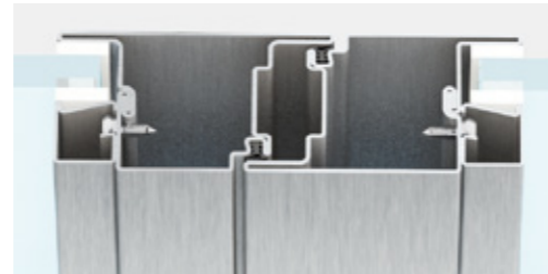
central section | frame section 151 mm
