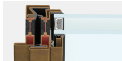
lateral section | frame section 47 mm
