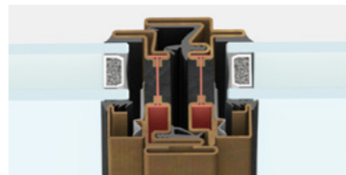
central section | frame section 62 mm
