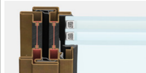
lateral section | frame section 47 mm
