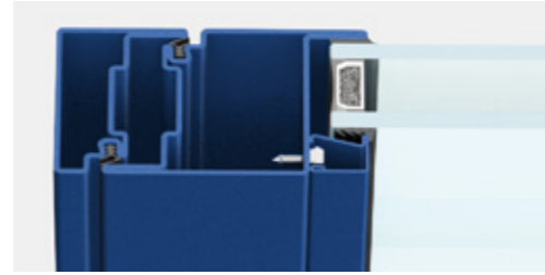
reduced lateral section | frame section 106 mm
