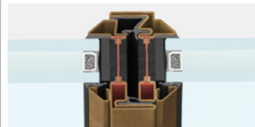
central section | frame section 62 mm
