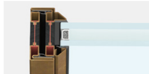
lateral section | frame section 47 mm
