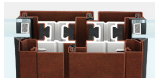
central section | frame section 156 mm
