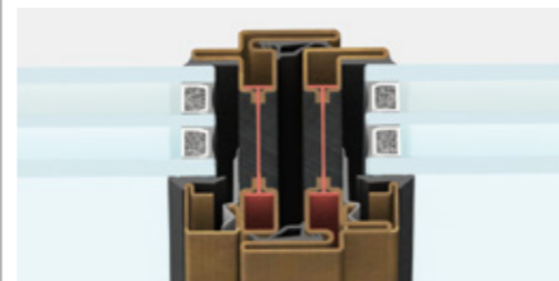
central section | frame section 62 mm
