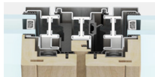
central section | frame section 145 mm
